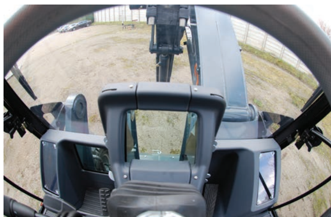
A fish-eye view through the steering wheel highlights the console's portals, which provide views of the wheels, as well as the bucket when digging right up to the machine
