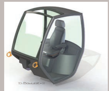
Early 3D concept sketches exploring the cab geometry and construction
